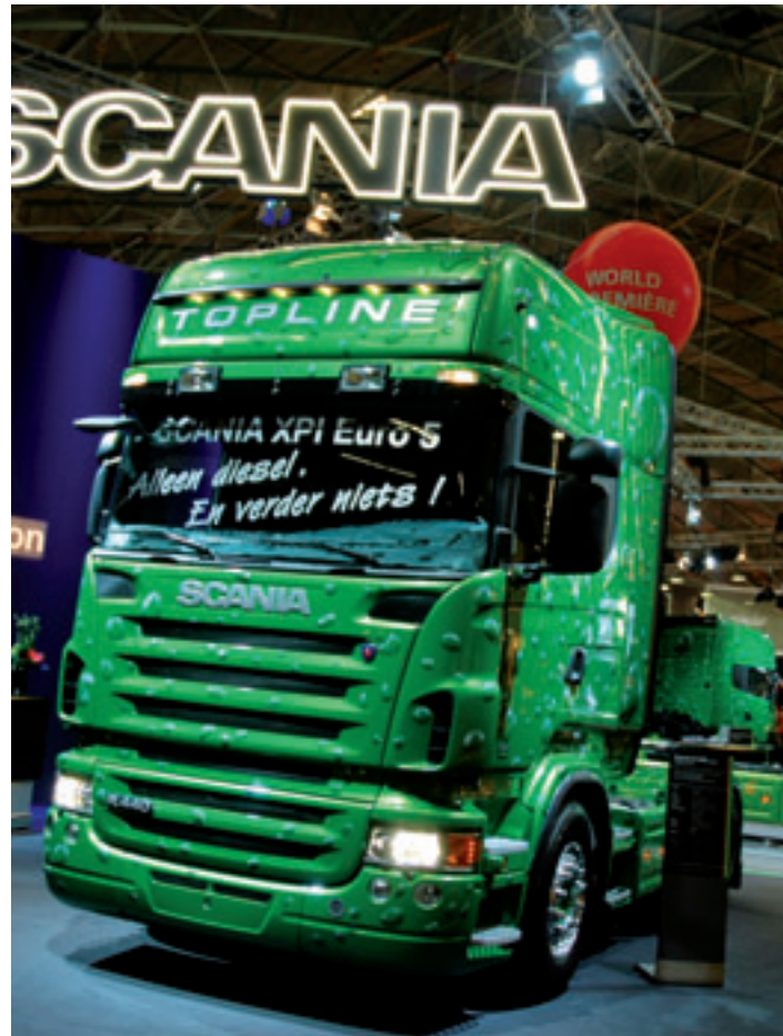
Scania is offering a complete range of Euro-5 engines using EGR technology.
